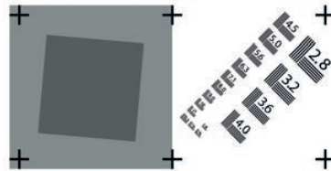
Figure C.10 — Example of slanted edges
