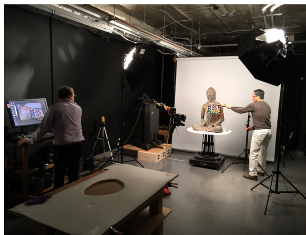
Figure 5 Scene-referred camera calibrations in preparation for a photogrammetric capture session to image the entire outside of the artwork
