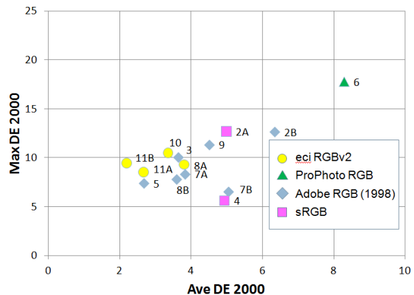
Figure 8. Plot of maximum versus average CIE DE2000 values for the ROIs on Print A.
